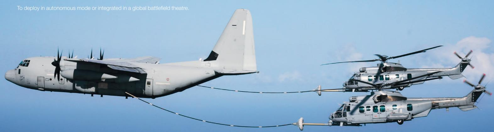
Unrivalled range with up to 3 tons of fuel tank capacity complemented by Air to Air Refueling (AAR), or Hover In Flight Refueling (HIFR) capabilities.
